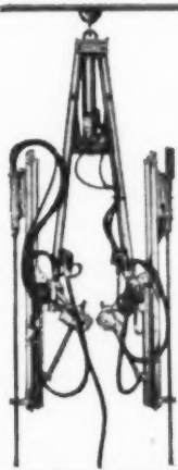
★ The SDR 34 shaft sinker for faster shaft sinking. Fully closed it's 5'6" between drill centers; open 19'3". All adjustments quickly made with air motor.
